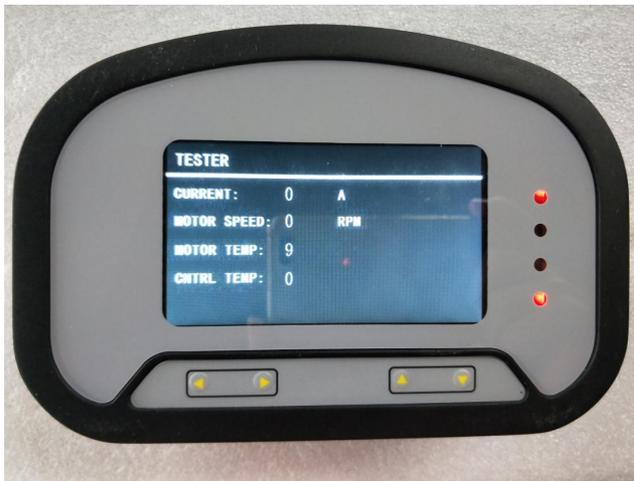
Entry method: With the cursor in "TESTER", press the ◀ key once to enter the second-level menu; the "TESTER" submenu includes "CURRENT (output current)", "MOTOR SPEED (motor speed)", "MOTOR TEMP (Motor temperature)", CNTRL TEMP (drive temperature).
