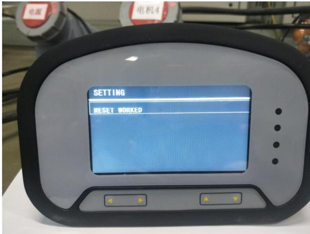
Entry method: In the case of the main interface, press **▶** once, then press **▼** again, move the cursor to SETTING, and then press **▶** to enter the hour meter clear input password interface, press **▲** key, enter the first password, and then press **▼** to enter into the second password change, input the four digit password in sequence, and press the **▶** confirm button to clear the hour meter.
