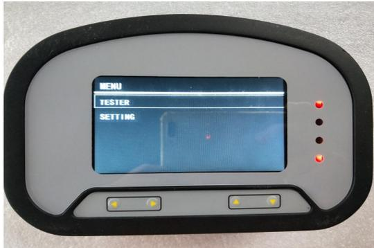
Entry method: In the case of the main interface, press ► key once to enter the first-level menu. The first-level menu includes the "TESTER" and "SETTING" second-level menus.
