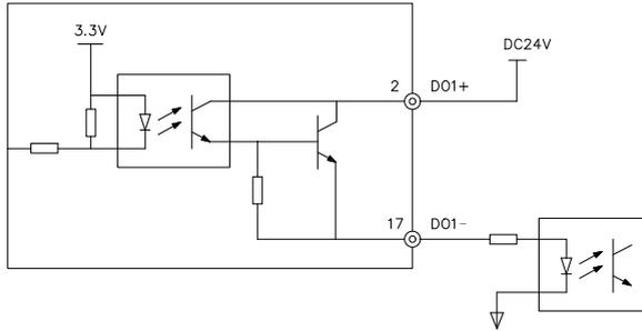
Fig.4-8 DO terminal source (PNP) output wiring mode
