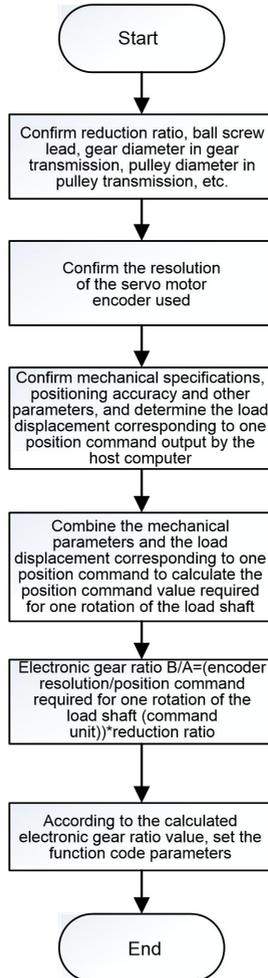
Fig.6-3 Electronic gear ratio setting process
