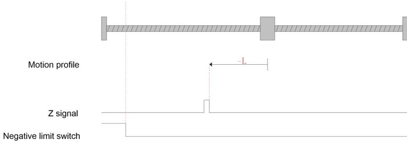
Fig.6-13 Homing mode 3 motion profile Figure 1
