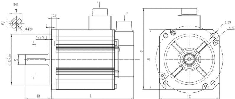
Fig.2-7 Dimensions for 130 frame medium inertia servo motor
