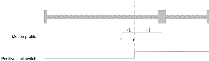
Fig.6-22 Homing mode 6 motion profile Figure 2
