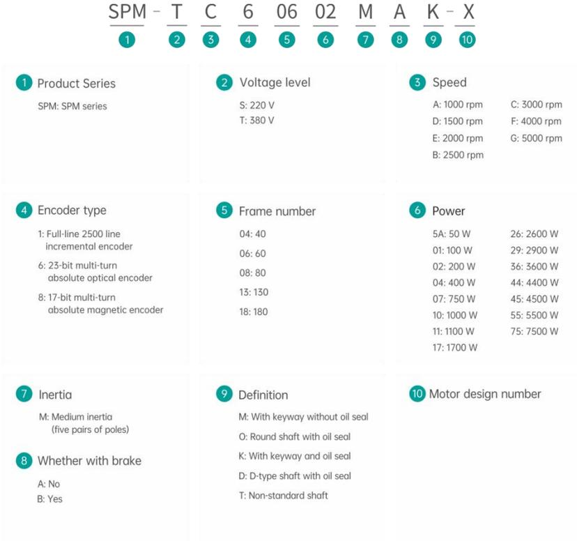
Fig.1-1 Servo motor model
