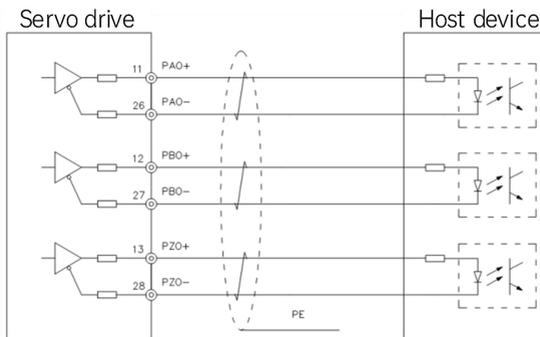
Fig.4-17 Encoder frequency dividing output wiring 2
