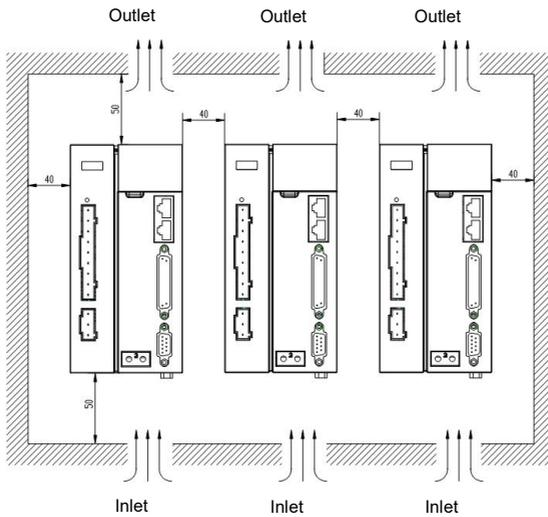
Fig.3-2 SIZE B/C servo installation diagram
