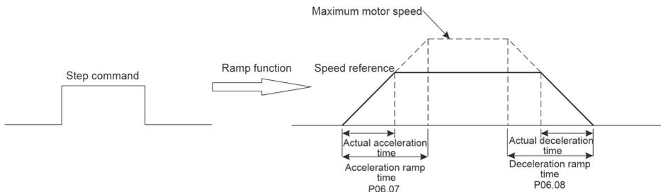
Fig.6-32 Command ramp function operating logic
