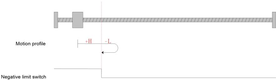
Fig.6-24 Homing mode 7 motion profile Figure 2
