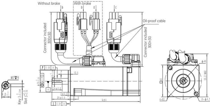
Fig.2-4 Dimensions for 40 frame medium inertia servo motor
