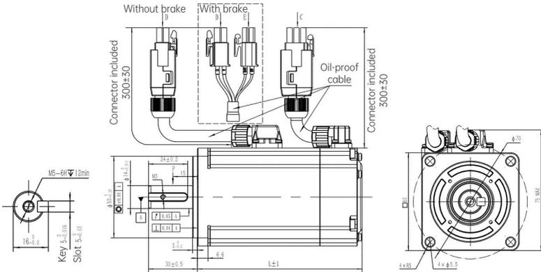
Fig.2-5 Dimensions for 60 frame medium inertia servo motor
