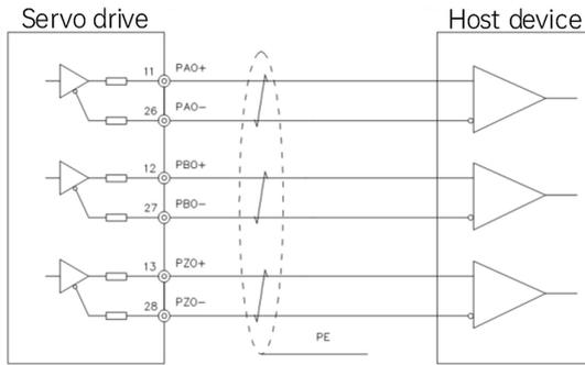
Fig.4-16 Encoder frequency dividing output wiring 1
