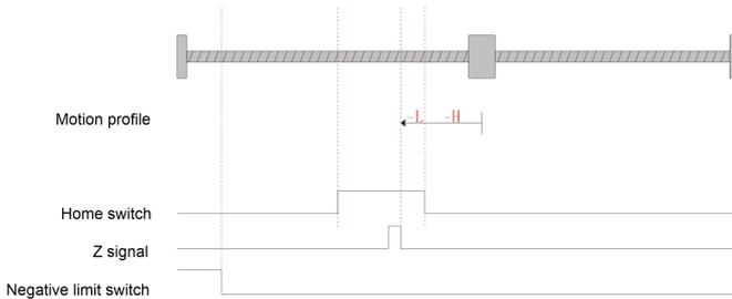
Fig.6-20 Homing mode 5 motion profile Figure 3
