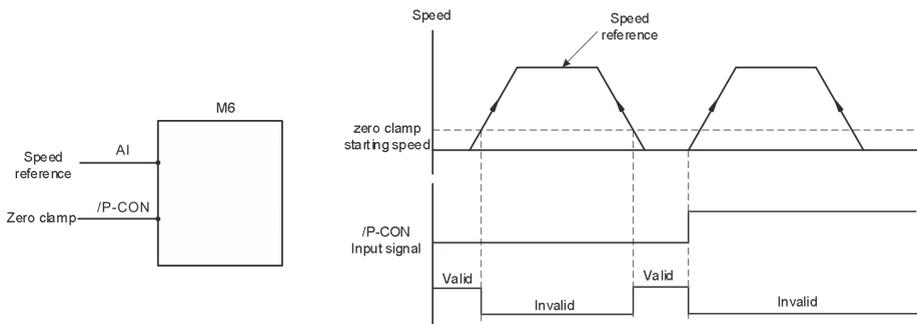
Fig.6-33 Zero clamp logic
