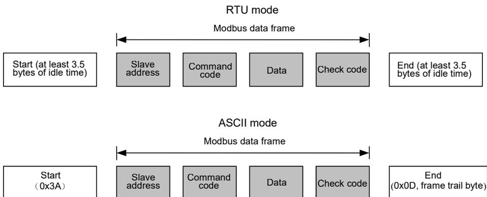
Attached Fig.1-1 Modbus protocol format
