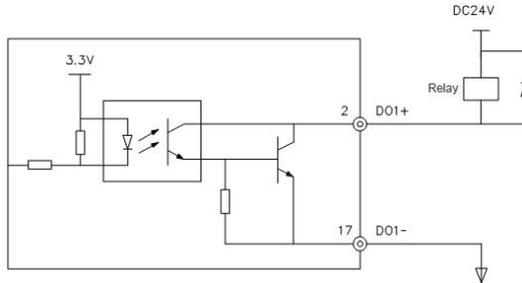
Fig.4-6 DO terminal connection relay wiring mode
