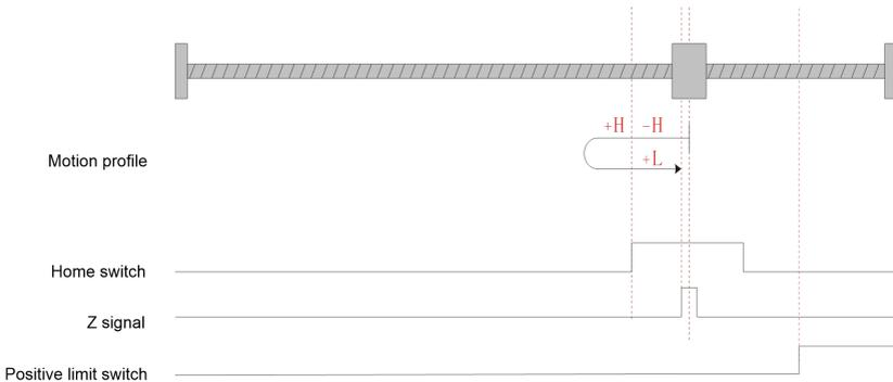
Fig.6-16 Homing mode 4 motion profile Figure 2
