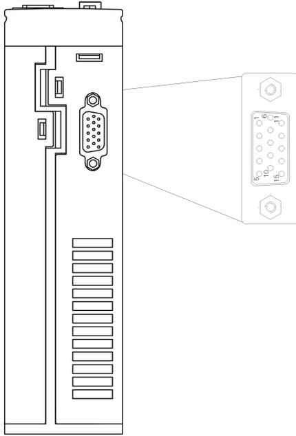
Fig.4-18 The second encoder signal connection diagram
