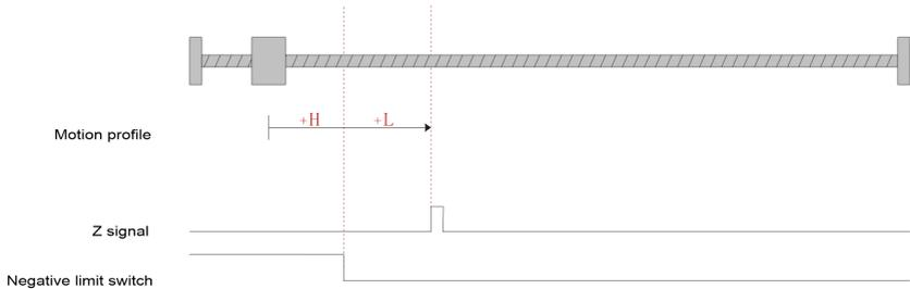
Fig.6-28 Homing mode 9 motion profile Figure 2
