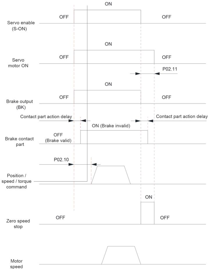
Fig.6-39 The brake timing when the servo motor is stationary
