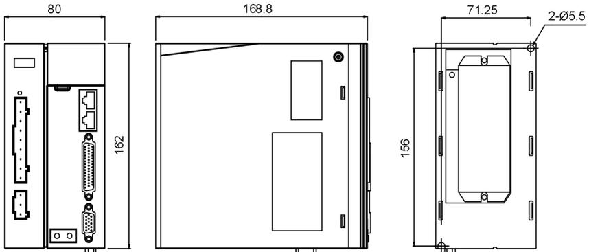
Fig.2-2 Dimensions for servo drive of SIZE B
