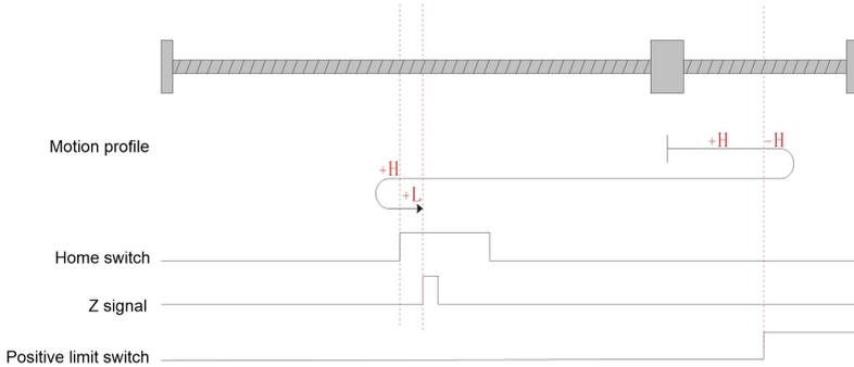
Fig.6-17 Homing mode 4 motion profile Figure 3
