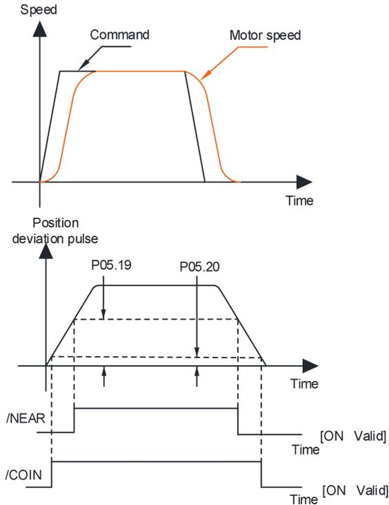
Fig.6-2 Positioning close to and positioning completed signal logic
