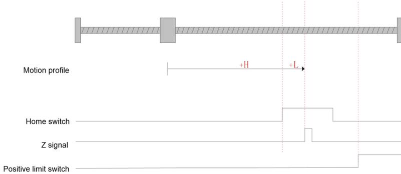
Fig.6-15 Homing mode 4 motion profile Figure 1
