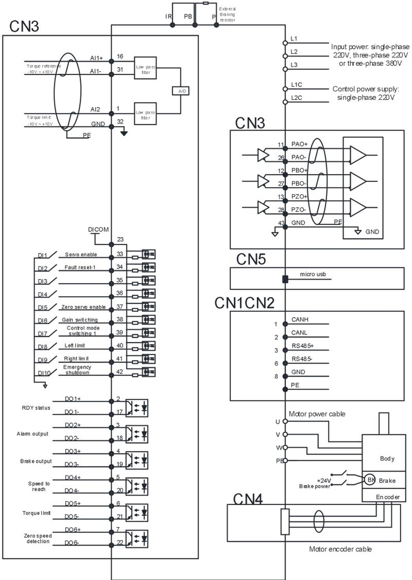
Fig.6-35 Torque control mode wiring
