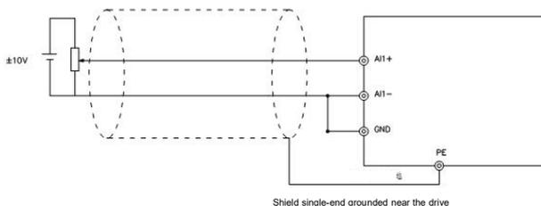
Fig.4-10 AI1 single-ended voltage input wiring diagram
