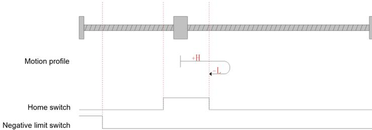
Fig.6-9 Homing mode 1 motion profile Figure 2
