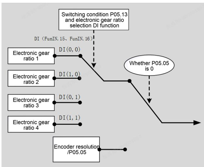
Fig.6-4 Electronic gear ratio function diagram
