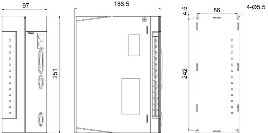
Fig.2-3 Dimensions for servo drive of SIZE C
