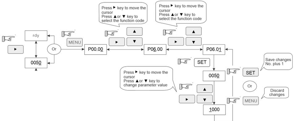
Fig.5-2 Working status display and parameter setting flowchart
