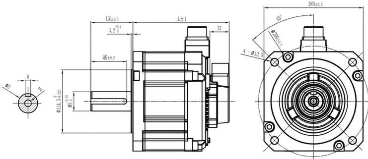
Fig.2-8 Dimensions for 180 frame medium inertia servo motor
