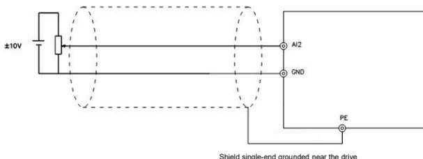
Fig.4-11 AI2 single-ended voltage input wiring diagram
