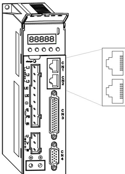
Fig.4-19 Communication interface connection diagram
