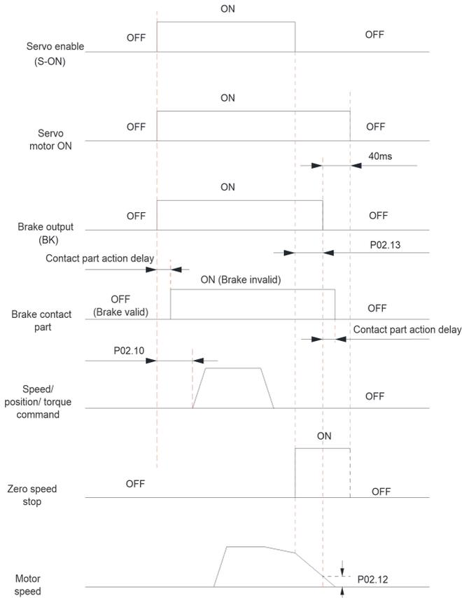
Fig.6-40 The brake timing when the servo motor is rotating
