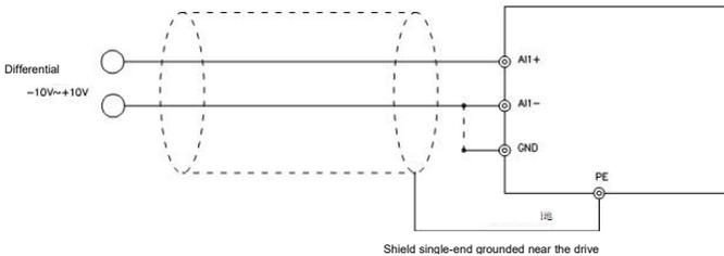
Fig.4-9 A11 differential voltage input wiring diagram
