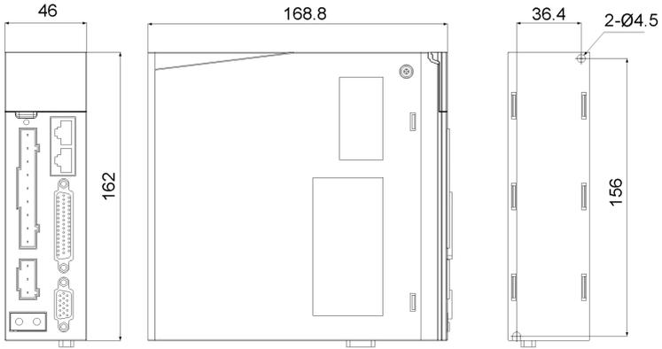
Fig.2-1 Dimensions for servo drive of SIZE A
