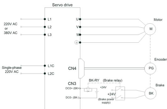
Fig.6-38 Brake wiring diagram
