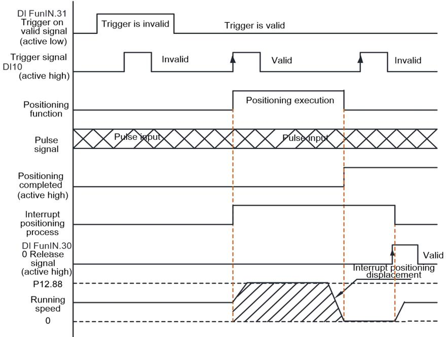
Fig.6-29 Interrupt positioning sequence diagram
