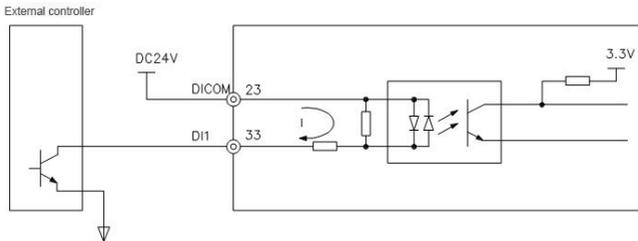
Fig.4-4 DI terminal NPN connection mode
