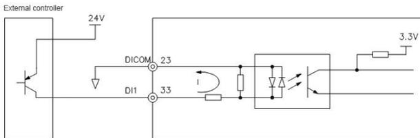
Fig.4-5 DI terminal PNP connection mode
