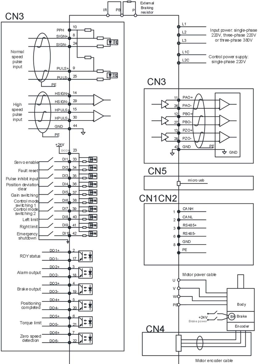
Fig.6-1 Position control mode wiring
