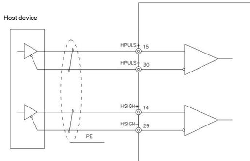
Fig.4-15 High-speed pulse input wiring diagram
