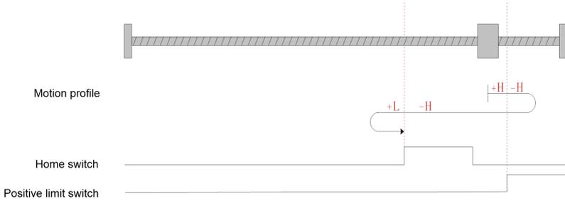
Fig.6-7 Homing mode 0 motion profile Figure 3
