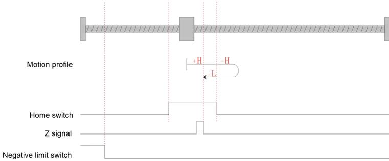
Fig.6-19 Homing mode 5 motion profile Figure 2
