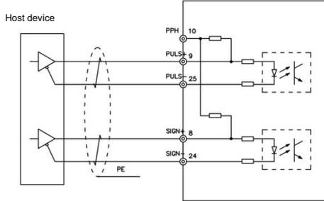
Fig.4-12 Low-speed pulse command differential input wiring diagram
