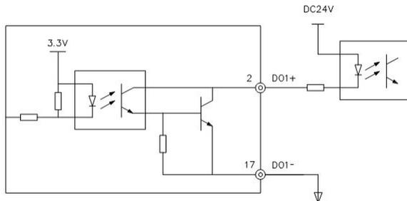
Fig.4-7 DO terminal drain (NPN) output wiring mode
