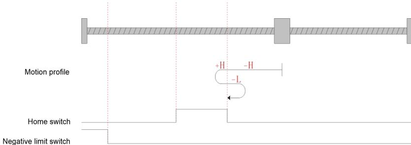
Fig.6-10 Homing mode 1 motion profile Figure 3
