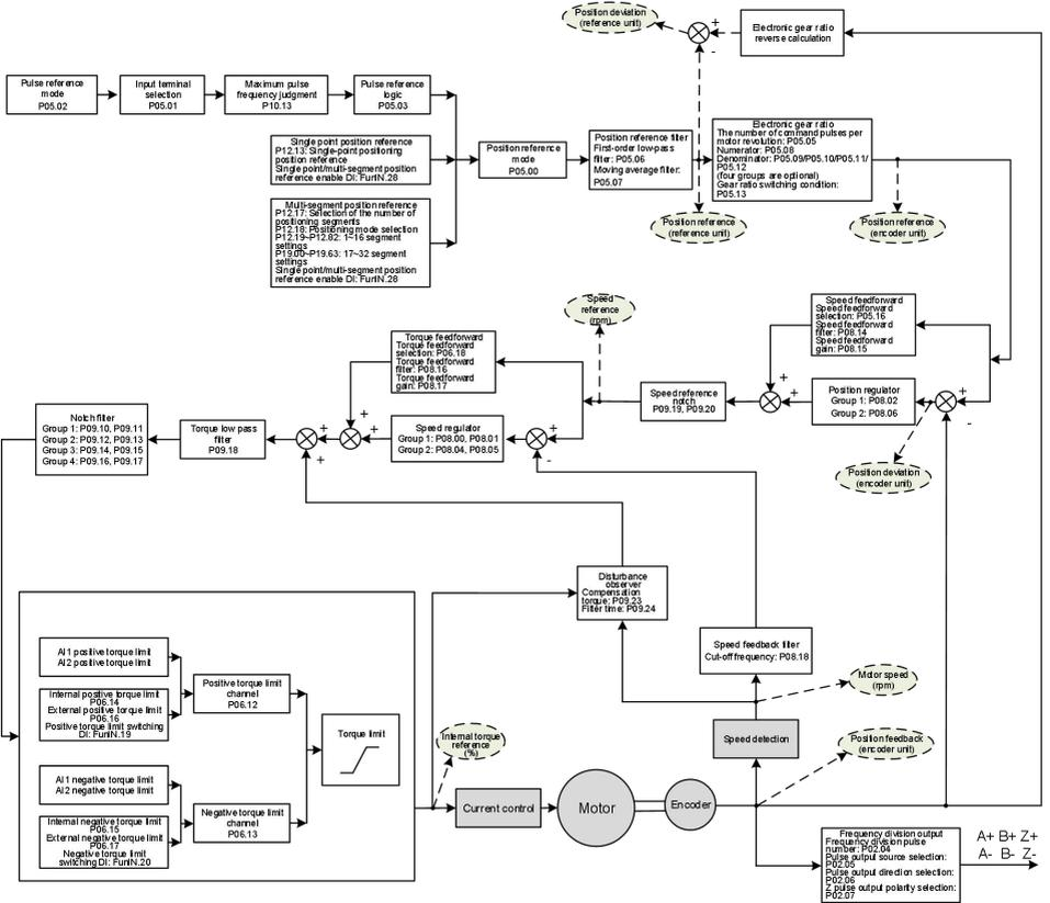
Fig.6-30 Function block diagram of position control mode
