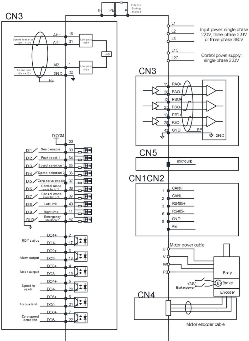
Fig.6-31 Speed control mode wiring
