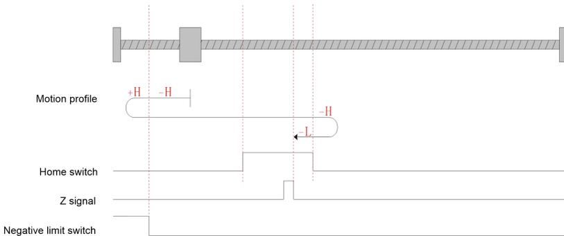
Fig.6-18 Homing mode 5 motion profile Figure 1
