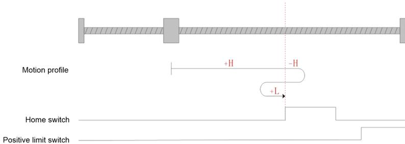
Fig.6-5 Homing mode 0 motion profile Figure 1
