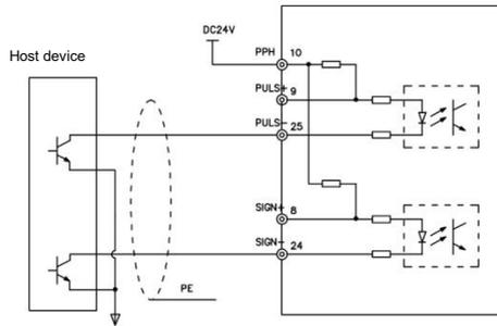
Fig.4-13 Low-speed pulse command NPN input wiring diagram
