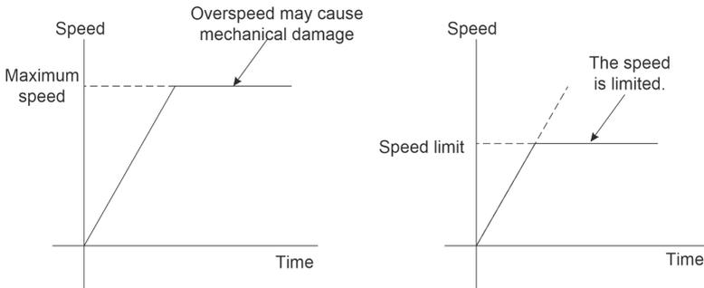
Fig.6-36 Speed limiter in torque control
